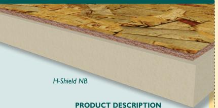
H-Shield NB is a rigid roof insulation composite panel composed of a closed cell polyisocyanurate foam core bonded during the manufacturing process to fiber reinforced facers on one side and either 7/16" or 5/8" oriented strand board (OSB) on the other. H-Shield NB can also be manufactured off-line using an FM approved adhesive.
